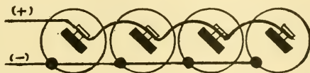
Fig. 61.—Diagram of a multiple or parallel connection. When connected in this manner the voltage of the battery is the same as that of a single cell, but the amperage of the battery is equal to the amperage of a single cell multiplied by the number of cells.
